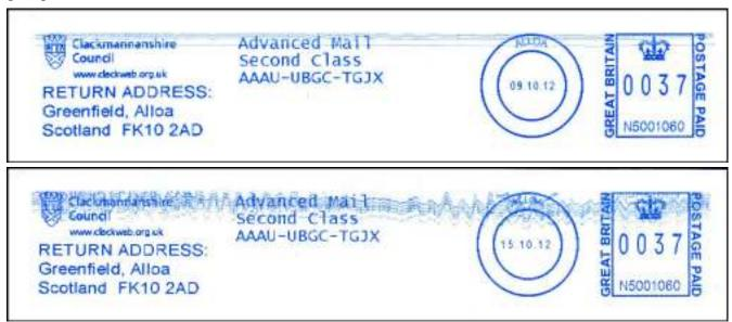
Further to page 116.5, here is another example of a MyMail frank where the top of the print has become increasingly separated from the lower half. The user later superimposed a second impression. The machine in question is FM2118505 (see the normal impression on page 134-11), whereas previously the error occurred on machine FM2118730. It appears, therefore, that a whole batch of machines may have been affected by this software error.
